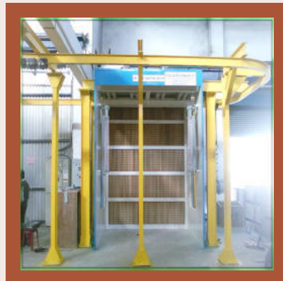
Dry Paint Booths
