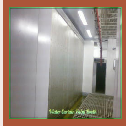
Conveyorised Water Wall Type Paint Booth
